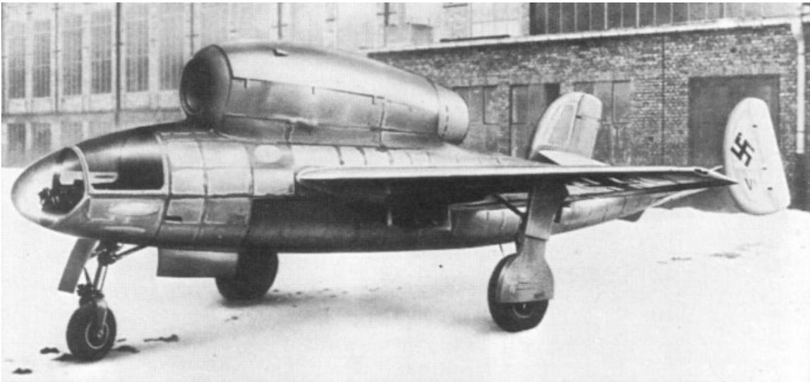
Henschel's **Hs 132** was a World War II dive bomber and interceptor aircraft of the German *Luftwaffe* that never saw service. The unorthodox design featured a top-mounted BMW 003 jet engine (identical in terms of make and position to the powerplant used by the Heinkel He 162) and the pilot in a prone position. The Soviet Army occupied the factory just as the **Hs 132 V1** was nearing flight testing, the **V2** and **V3** being 80% and 75% completed.
