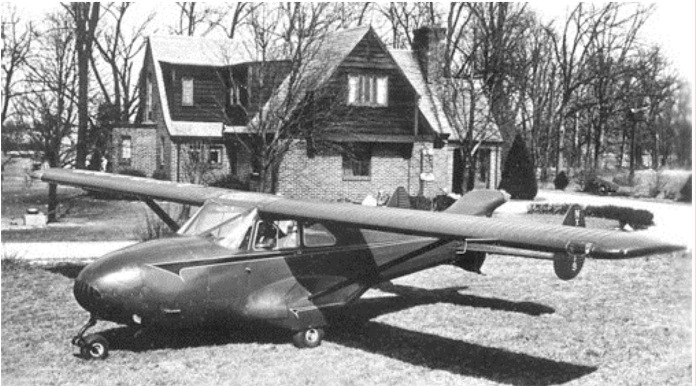
The **Waco Model W Aristocraft** was an American four-seat monoplane, the last aircraft designed and built by the Waco Aircraft Company. It had an unusual configuration with an engine mounted at the front driving a pusher propeller at the rear.
