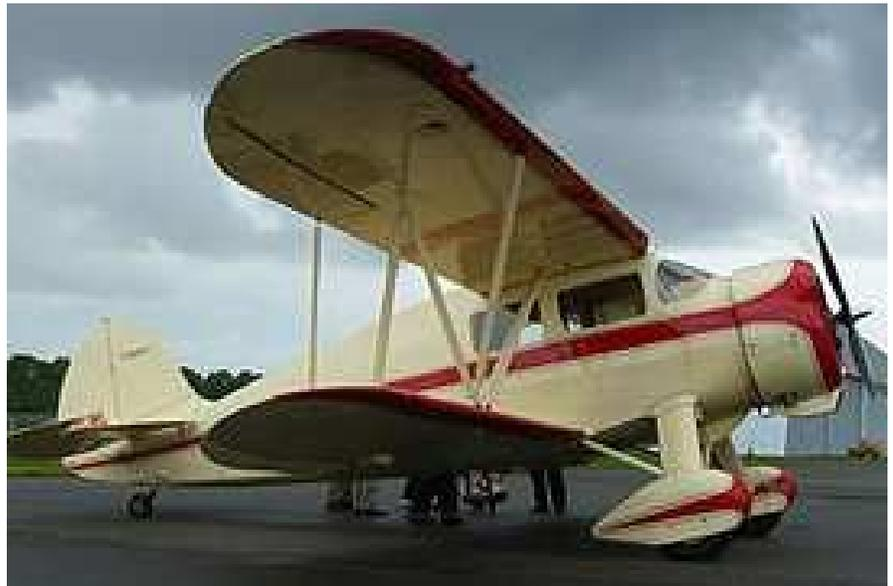
spars with the airfoil formed from trussed ribs made from plywood and spruce. The leading edge
