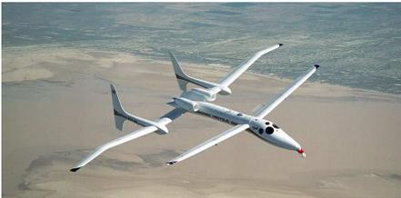
payloads on a ventral pylon. An extremely efficient design, the Proteus can orbit a point at over 65,000 feet
